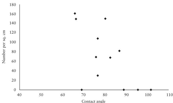
**Figure 4.1** Number of macrofoulers at the end of three days placement, on polyvinyl chloride, PP, HDPE, PC, GFRP, Teflon®, SF, acrylic, silicone, PU, polydimethylsiloxane (PDMS) and polyester (correlation coefficient = 0.60)
