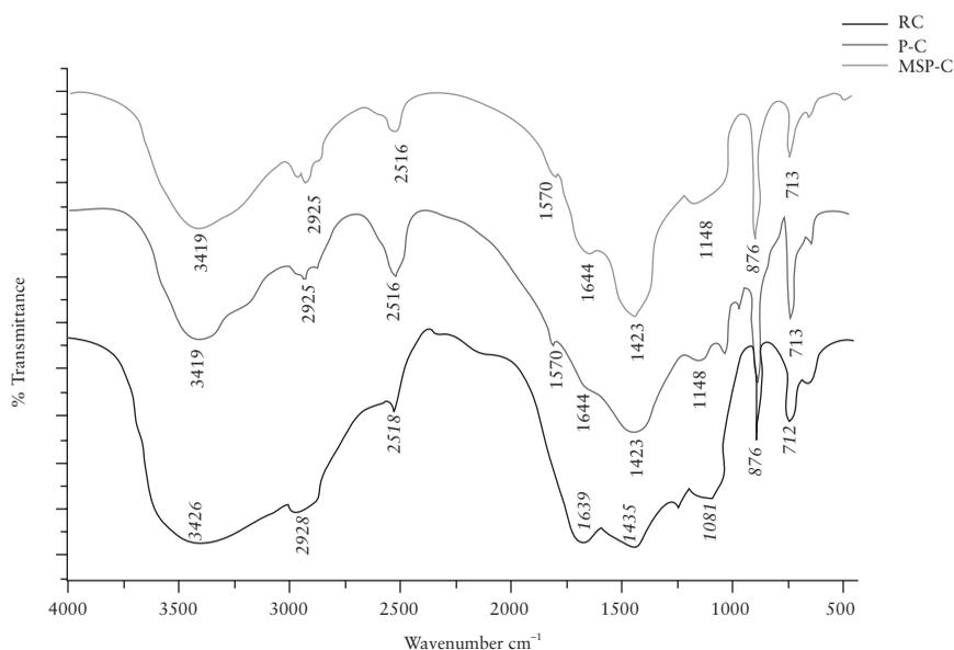
**Figure 4.3** FTIR spectra of cements collected from barnacle, *A. reticulatus* attached on different substrates. RC: Rubber like cement from barnacle attached on mussel shell (thick and opaque), P-C: powder like cement from a barnacle attached on PMMA (thin and transparent) and MSP-C: powder like cement from a barnacle attached to a mussel shell
