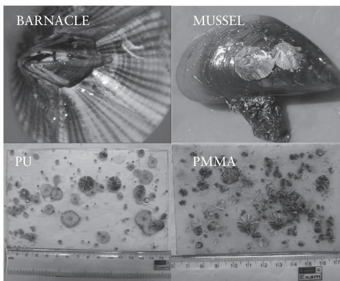
**Figure 4.2** Barnacles attached to PU, polymethyl methacrylate (PMMA) and mussel surfaces placed in the ocean for one year.
